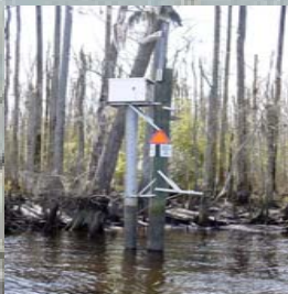
Figure 2. Data collection platform recording water level and salinity every six seconds.
