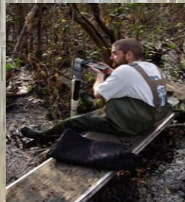
Water level instrument being downloaded at a subsite within a belt transect.
